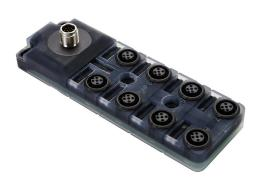
Exact 12 passive distribution block, 8 ports, 5-pin M12 sockets, (2) 5-wire and (6) 4-wire, 24 VDC, 1A, power and PNP LED indicator(s), 12-pin M12 quick-disconnect, IP67. Marking tags included.
