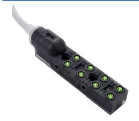
Exact 8 passive distribution block, 8 ports, 4-pin M8 sockets, 4-wire, 24 VDC, 2A, power and NPN LED indicator(s), 5m integrated cable, IP67. Marking tags included.
