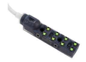
Exact 8 passive distribution block, 8 ports, 4-pin M8 sockets, 4-wire, 24 VDC, 2A, power and PNP LED indicator(s), 5m integrated cable, IP67. Marking tags included.
