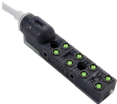
Exact 8 passive distribution block, 8 ports, 3-pin M8 sockets, 3-wire, 24 VDC, 2A, power and NPN LED indicator(s), 5m integrated cable, IP67. Marking tags included.
