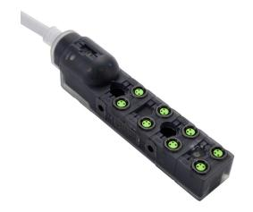
Exact 8 passive distribution block, 8 ports, 3-pin M8 sockets, 3-wire, 24 VDC, 2A, power and NPN LED indicator(s), 5m integrated cable, IP67. Marking tags included.
