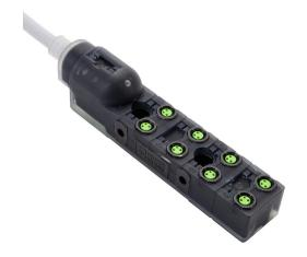
Exact 8 passive distribution block, 8 ports, 3-pin M8 sockets, 3-wire, 24 VDC, 2A, power and PNP LED indicator(s), 5m integrated cable, IP67. Marking tags included.
