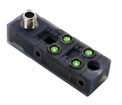
Exact 8 passive distribution block, 4 ports, 4-pin M8 sockets, 4-wire, 24 VDC, 1A, power and PNP LED indicator(s), 12-pin M12 quick-disconnect, IP67. Marking tags included.
