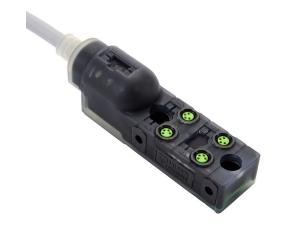
Exact 8 passive distribution block, 4 ports, 4-pin M8 sockets, 4-wire, 24 VDC, 2A, power and NPN LED indicator(s), 5m integrated cable, IP67. Marking tags included.
