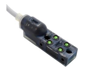
Exact 8 passive distribution block, 4 ports, 4-pin M8 sockets, 4-wire, 24 VDC, 2A, power and PNP LED indicator(s), 5m integrated cable, IP67. Marking tags included.
