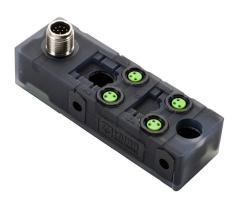
Exact 8 passive distribution block, 4 ports, 3-pin M8 sockets, 3-wire, 24 VDC, 1A, power and PNP LED indicator(s), 12-pin M12 quick-disconnect, IP67. Marking tags included.
