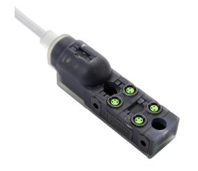
Exact 8 passive distribution block, 4 ports, 3-pin M8 sockets, 3-wire, 24 VDC, 2A, power and NPN LED indicator(s), 5m integrated cable, IP67. Marking tags included.
