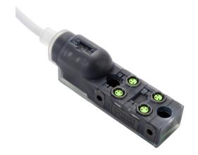
Exact 8 passive distribution block, 4 ports, 3-pin M8 sockets, 3-wire, 24 VDC, 2A, power and PNP LED indicator(s), 5m integrated cable, IP67. Marking tags included.
