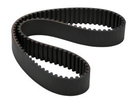
SureMotion timing belt, 8mm 8M pitch, 30mm wide, 100 tooth, 800mm pitch length (circumference), neoprene, fiberglass reinforced.
