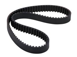
SureMotion timing belt, 8mm 8M pitch, 20mm wide, 100 tooth, 800mm pitch length (circumference), neoprene, fiberglass reinforced.
