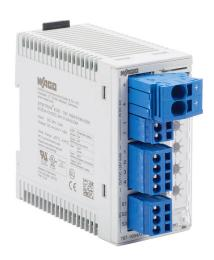
WAGO electronic circuit protector, adjustable 1-6A, 24 VDC, 4 independent channel(s), 35mm DIN rail mount.
