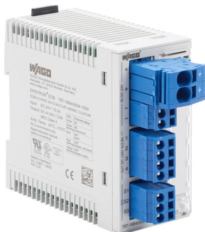
WAGO electronic circuit protector, current-limiting, 3.8A, 24 VDC, 4 independent channel(s), NEC Class 2, 35mm DIN rail mount.
