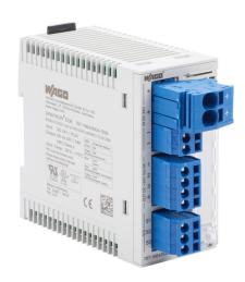
WAGO electronic circuit protector, current-limiting, 3.8A, 24 VDC, 4 independent channel(s), NEC Class 2, 35mm DIN rail mount.
