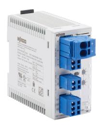
WAGO electronic circuit protector, current-limiting, adjustable 0.5-6A, 24 VDC, 2 independent channel(s), 35mm DIN rail mount.
