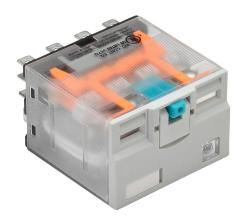
AutomationDirect ice cube control relay, socket mount, encapsulated push-to-test, 12 VDC coil voltage, 4PDT, (4) N.O., (4) N.C., 15A contact rating, 14-pin, LED indicator(s). Requires 784-4C-SKT-1 mounting socket.
