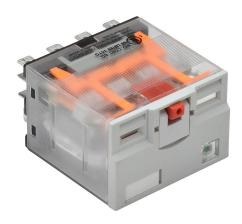
AutomationDirect ice cube control relay, socket mount, encapsulated push-to-test, 12 VAC coil voltage, 4PDT, (4) N.O., (4) N.C., 15A contact rating, 14-pin, LED indicator(s). Requires 784-4C-SKT-1 mounting socket.
