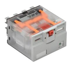
AutomationDirect ice cube control relay, socket mount, encapsulated push-to-test, 12 VAC coil voltage, 4PDT, (4) N.O., (4) N.C., 15A contact rating, 14-pin, LED indicator(s). Requires 784-4C-SKT-1 mounting socket.
