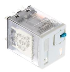
AutomationDirect ice cube control relay, socket mount, encapsulated push-to-test, 24 VDC coil voltage, 3PDT, (3) N.O., (3) N.C., 15A contact rating, 11-pin, LED indicator(s). Requires 783-3C-SKT mounting socket.
