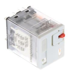
AutomationDirect ice cube control relay, socket mount, encapsulated push-to-test, 24 VAC coil voltage, 3PDT, (3) N.O., (3) N.C., 15A contact rating, 11-pin, LED indicator(s). Requires 783-3C-SKT mounting socket.
