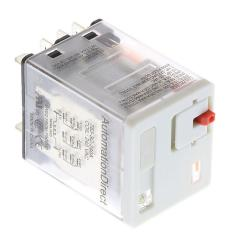
AutomationDirect ice cube control relay, socket mount, encapsulated push-to-test, 240 VAC coil voltage, 3PDT, (3) N.O., (3) N.C., 15A contact rating, 11-pin, LED indicator(s). Requires 783-3C-SKT mounting socket.
