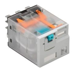
AutomationDirect ice cube control relay, socket mount, encapsulated push-to-test, 12 VDC coil voltage, 3PDT, (3) N.O., (3) N.C., 15A contact rating, 11-pin, LED indicator(s). Requires 783-3C-SKT mounting socket.
