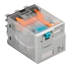
AutomationDirect ice cube control relay, socket mount, encapsulated push-to-test, 12 VDC coil voltage, 3PDT, (3) N.O., (3) N.C., 15A contact rating, 11-pin, LED indicator(s). Requires 783-3C-SKT mounting socket.
