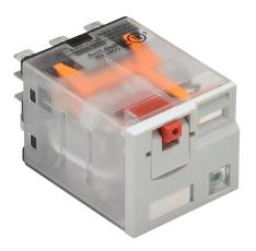
AutomationDirect ice cube control relay, socket mount, encapsulated push-to-test, 12 VAC coil voltage, 3PDT, (3) N.O., (3) N.C., 15A contact rating, 11-pin, LED indicator(s). Requires 783-3C-SKT mounting socket.
