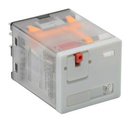
AutomationDirect ice cube control relay, socket mount, encapsulated push-to-test, 120 VAC coil voltage, 3PDT, (3) N.O., (3) N.C., 15A contact rating, 11-pin, LED indicator(s). Requires 783-3C-SKT mounting socket.
