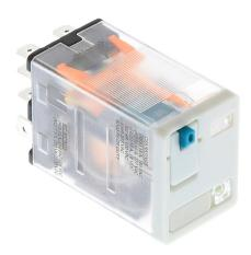
AutomationDirect ice cube control relay, socket mount, encapsulated push-to-test, 24 VDC coil voltage, DPDT, (2) N.O., (2) N.C., 15A contact rating, 8-pin, LED indicator(s). Requires 782-2C-SKT mounting socket.
