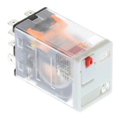
AutomationDirect ice cube control relay, socket mount, encapsulated push-to-test, 24 VAC coil voltage, DPDT, (2) N.O., (2) N.C., 15A contact rating, 8-pin, LED indicator(s). Requires 782-2C-SKT mounting socket.
