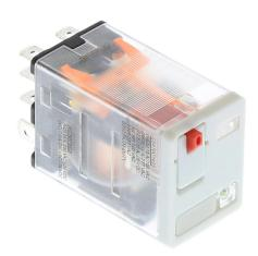
AutomationDirect ice cube control relay, socket mount, encapsulated push-to-test, 240 VAC coil voltage, DPDT, (2) N.O., (2) N.C., 15A contact rating, 8-pin, LED indicator(s). Requires 782-2C-SKT mounting socket.
