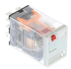
AutomationDirect ice cube control relay, socket mount, encapsulated push-to-test, 240 VAC coil voltage, DPDT, (2) N.O., (2) N.C., 15A contact rating, 8-pin, LED indicator(s). Requires 782-2C-SKT mounting socket.
