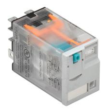
AutomationDirect ice cube control relay, socket mount, encapsulated push-to-test, 12 VDC coil voltage, DPDT, (2) N.O., (2) N.C., 15A contact rating, 8-pin, LED indicator(s). Requires 782-2C-SKT mounting socket.
