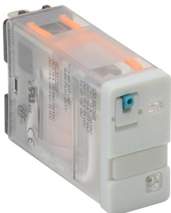
AutomationDirect ice cube control relay, socket mount, encapsulated push-to-test, 24 VDC coil voltage, SPDT, (1) N.O., (1) N.C., 15A contact rating, 5-pin, LED indicator(s). Requires 781-1C-SKT mounting socket.
