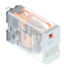
AutomationDirect ice cube control relay, socket mount, encapsulated push-to-test, 240 VAC coil voltage, SPDT, (1) N.O., (1) N.C., 15A contact rating, 5-pin, LED indicator(s). Requires 781-1C-SKT mounting socket.
