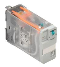
AutomationDirect ice cube control relay, socket mount, encapsulated push-to-test, 12 VDC coil voltage, SPDT, (1) N.O., (1) N.C., 15A contact rating, 5-pin, LED indicator(s). Requires 781-1C-SKT mounting socket.
