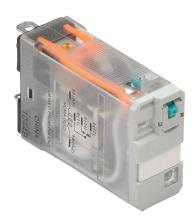
AutomationDirect ice cube control relay, socket mount, encapsulated push-to-test, 12 VDC coil voltage, SPDT, (1) N.O., (1) N.C., 15A contact rating, 5-pin, LED indicator(s). Requires 781-1C-SKT mounting socket.
