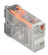
AutomationDirect ice cube control relay, socket mount, encapsulated push-to-test, 12 VAC coil voltage, SPDT, (1) N.O., (1) N.C., 15A contact rating, 5-pin, LED indicator(s). Requires 781-1C-SKT mounting socket.
