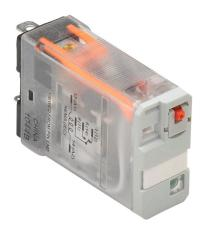
AutomationDirect ice cube control relay, socket mount, encapsulated push-to-test, 12 VAC coil voltage, SPDT, (1) N.O., (1) N.C., 15A contact rating, 5-pin, LED indicator(s). Requires 781-1C-SKT mounting socket.
