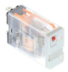
AutomationDirect ice cube control relay, socket mount, encapsulated push-to-test, 120 VAC coil voltage, SPDT, (1) N.O., (1) N.C., 15A contact rating, 5-pin, LED indicator(s). Requires 781-1C-SKT mounting socket.
