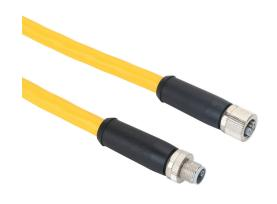
Murrelektronik power cable, M12 axial male L-coded to M12 axial female L-coded, 5-pole, 63 VDC, 16A, 14 AWG, TPE jacket, yellow, 32.8ft/10m cable length, IP65 IP67.
