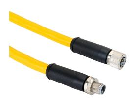
Murrelektronik power cable, M12 axial male L-coded to M12 axial female L-coded, 5-pole, 63 VDC, 16A, 14 AWG, TPE jacket, yellow, 24.6ft/7.5m cable length, IP65 IP67.
