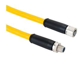
Murrelektronik power cable, M12 axial male L-coded to M12 axial female L-coded, 5-pole, 63 VDC, 16A, 14 AWG, TPE jacket, yellow, 16.4ft/5m cable length, IP65 IP67.
