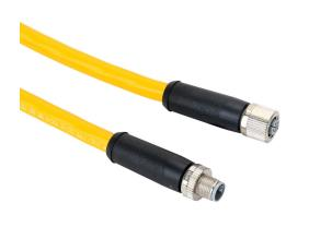
Murrelektronik power cable, M12 axial male L-coded to M12 axial female L-coded, 5-pole, 63 VDC, 16A, 14 AWG, TPE jacket, yellow, 9.8ft/3m cable length, IP65 IP67.
