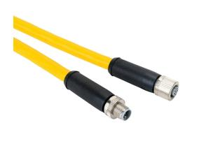
Murrelektronik power cable, M12 axial male L-coded to M12 axial female L-coded, 5-pole, 63 VDC, 16A, 14 AWG, TPE jacket, yellow, 6.5ft/2m cable length, IP65 IP67.
