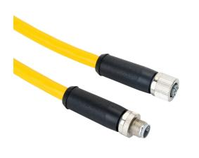
Murrelektronik power cable, M12 axial male L-coded to M12 axial female L-coded, 5-pole, 63 VDC, 12A, 16 AWG, TPE jacket, yellow, 16.4ft/5m cable length, IP65 IP67.
