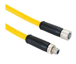
Murrelektronik power cable, M12 axial male L-coded to M12 axial female L-coded, 5-pole, 63 VDC, 12A, 16 AWG, TPE jacket, yellow, 9.8ft/3m cable length, IP65 IP67.
