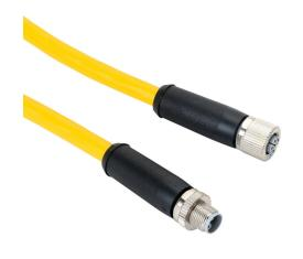
Murrelektronik power cable, M12 axial male L-coded to M12 axial female L-coded, 5-pole, 63 VDC, 12A, 16 AWG, TPE jacket, yellow, 6.5ft/2m cable length, IP65 IP67.
