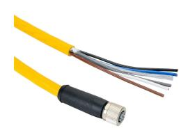
Murrelektronik power cable, M12 axial female L-coded to pigtail, 5-pole, 63 VDC, 16A, 14 AWG, TPE jacket, yellow, 49.2ft/15m cable length, IP65 IP67.
