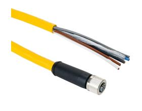
Murrelektronik power cable, M12 axial female L-coded to pigtail, 5-pole, 63 VDC, 16A, 14 AWG, TPE jacket, yellow, 32.8ft/10m cable length, IP65 IP67.
