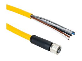
Murrelektronik power cable, M12 axial female L-coded to pigtail, 5-pole, 63 VDC, 16A, 14 AWG, TPE jacket, yellow, 32.8ft/10m cable length, IP65 IP67.
