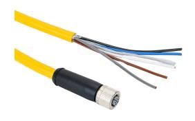
Murrelektronik power cable, M12 axial female L-coded to pigtail, 5-pole, 63 VDC, 12A, 16 AWG, TPE jacket, yellow, 49.2ft/15m cable length, IP65 IP67.
