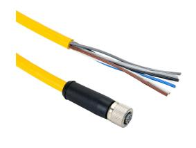
Murrelektronik power cable, M12 axial female L-coded to pigtail, 5-pole, 63 VDC, 12A, 16 AWG, TPE jacket, yellow, 24.6ft/7.5m cable length, IP65 IP67.
