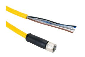
Murrelektronik power cable, M12 axial female L-coded to pigtail, 5-pole, 63 VDC, 12A, 16 AWG, TPE jacket, yellow, 16.4ft/5m cable length, IP65 IP67.
