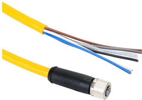
Murrelektronik power cable, M12 axial female L-coded to pigtail, 5-pole, 63 VDC, 12A, 16 AWG, TPE jacket, yellow, 9.8ft/3m cable length, IP65 IP67.
