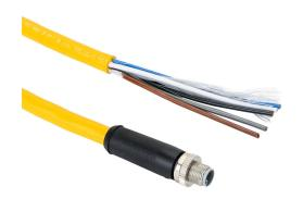
Murrelektronik power cable, M12 axial male L-coded to pigtail, 5-pole, 63 VDC, 16A, 14 AWG, TPE jacket, yellow, 32.8ft/10m cable length, IP65 IP67.
