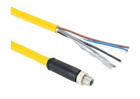
Murrelektronik power cable, M12 axial male L-coded to pigtail, 5-pole, 63 VDC, 16A, 14 AWG, TPE jacket, yellow, 24.6ft/7.5m cable length, IP65 IP67.
