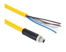
Murrelektronik power cable, M12 axial male L-coded to pigtail, 5-pole, 63 VDC, 16A, 14 AWG, TPE jacket, yellow, 9.8ft/3m cable length, IP65 IP67.
